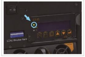
**STEP 3:** Please set desired parameters on replacement CE-R1, or the settings will follow factory default value when inserting new control unit.
