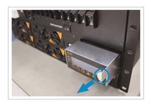
STEP 2: Insert the replacement control unit fully into the shelf (顯示方向) until it fits the slot tightly. Wait for few seconds until the LED on replacement CE-R1 shows solid GREEN.
