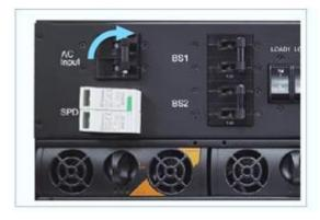
After power ON 5 to 10 sec. Please check CE-R1 LED green light is ON. And no alarm message. Please check CE-R1 display condition: normal.
