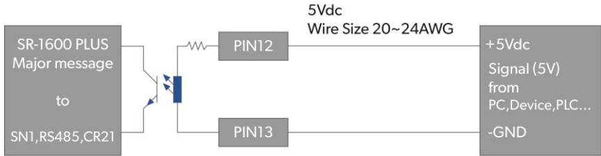
Figure 6-3. Application diagram of dry contact pin12~13(Major)
