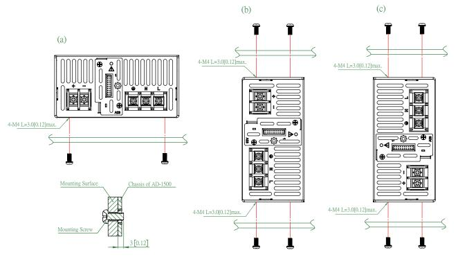
Recommended screw length is measured from the power supply surface
