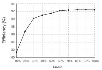
The curve above is measured at 230Vac (Ambient temperature @  $25^{\circ}$ C)
