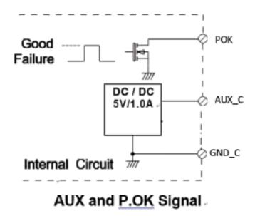
Open drain signal low when PSU turns on, Max. P.OK sink current: 20mA, Max. drain voltage: 40V
