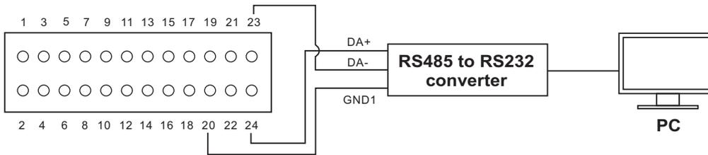
Note: Make sure GND1 (pin 20) is connected to the external communication kit when using RS485 / I<sup>2</sup>C
