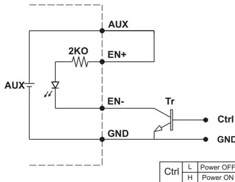
(B) ON / OFF Control by NPN transistor
