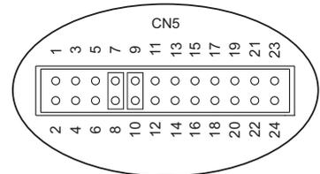
Control pin number assignment (CN5): JST S24B-PHDSS or equivalent
