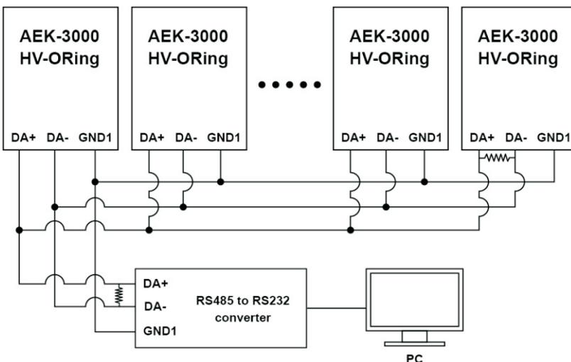
Note: Make sure GND1 (pin 20) is connected to the external communication kit when using RS485 / I<sup>2</sup>C
