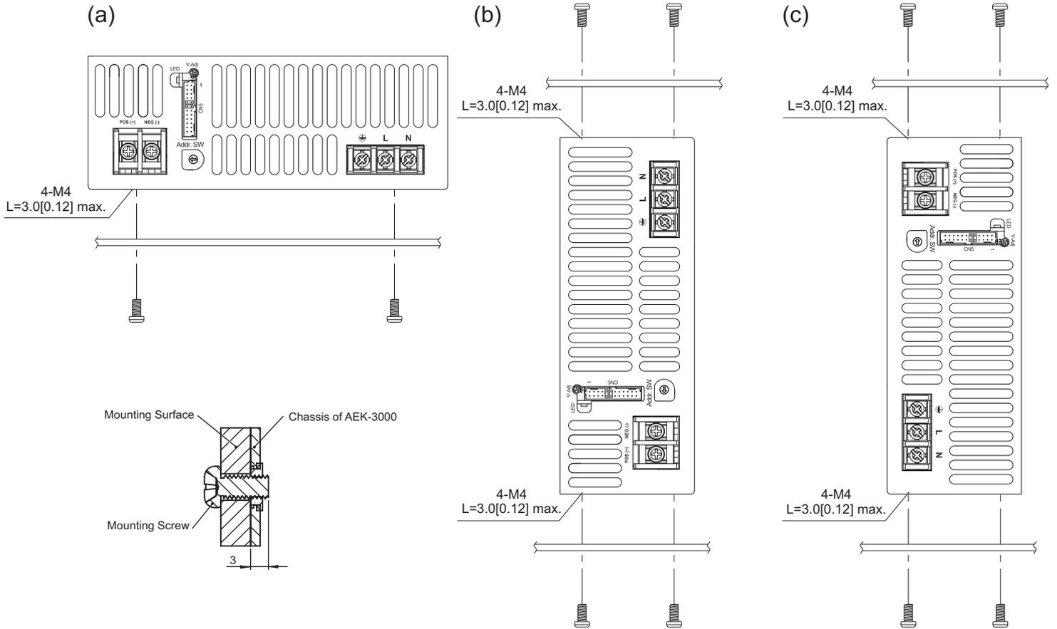
Recommended screw length is measured from the power supply surface
