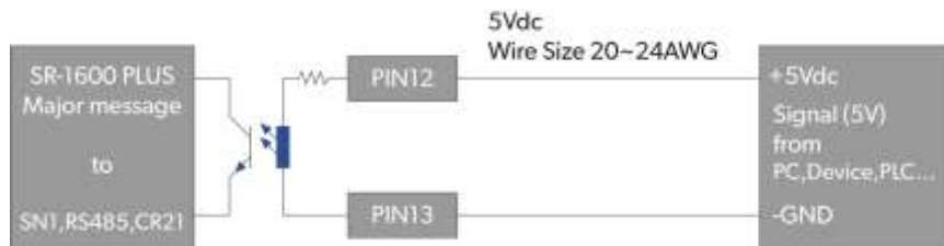
Figure 6-3. Application diagram of dry contact pin12~13(Major)
