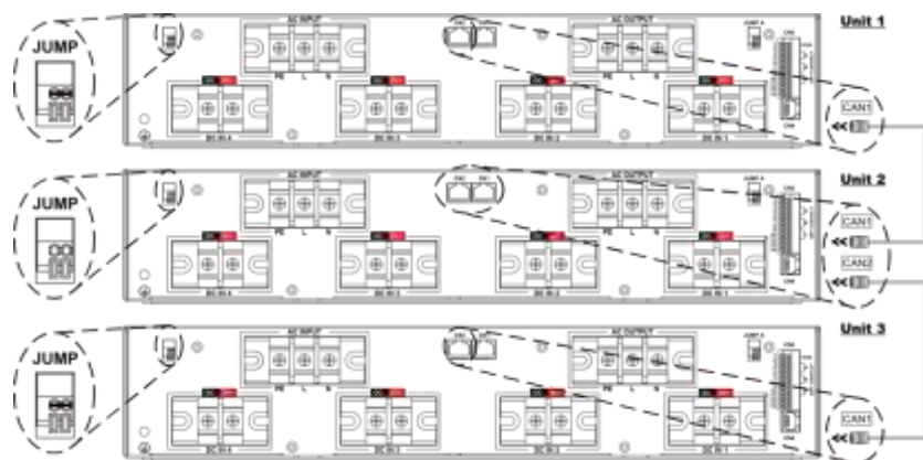
Figure 7-3. Parallel connection via jumper setting
