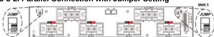
Figure 7-1. Parallel connection via jumper setting
